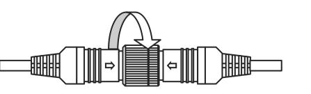
**3. Tighten cable connection firmly** in order to prevent water ingress.
